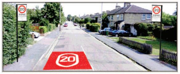
Example of how entry into the proposed limit on a smaller road could look with a 20mph roundel road marking and 20mph limit signs
